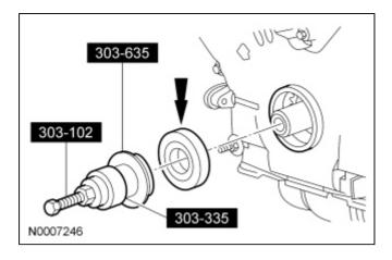
3. Install the crankshaft pulley. For additional information, refer to Crankshaft Pulley in this section.
