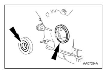
2. Using the Crankshaft Vibration Damper Installer, Front Cover Oil Seal Installer and the Crankshaft Front Oil Seal Installer, install the crankshaft front seal.
